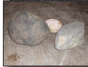
Rocks, such as these, at left, can cause a sewer spill, like the one pictured above.
